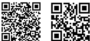
Figure 3: An example of a QR code containing a long URL (left) and a short URL (right). The short url is www.printing.org and the long URL is http://efiles.printing.org/eweb/docs/workshops/AgendaCM4P.pdf .
